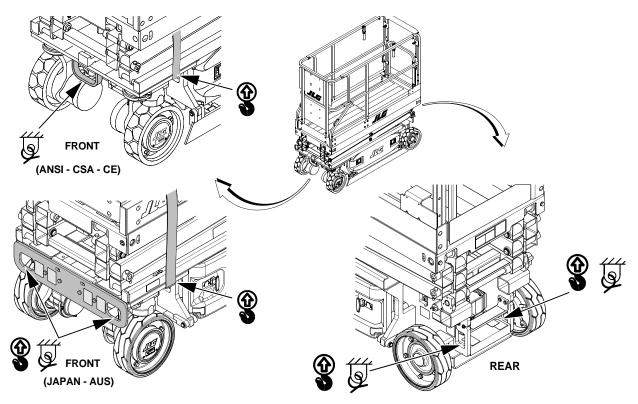
Figure 4-3. Lifting and Tie Down Diagram
