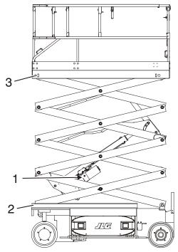
Figure 6-1. Lubrication Diagram
