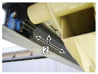
Figure 6-3. Upper Slide Pad Channel
