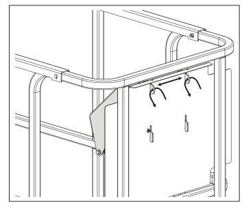
Figure 4-2. Securing Control Station to Platform
