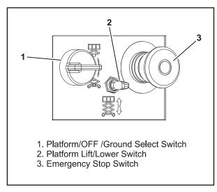
**Figure 3-1. Ground Control Station**
