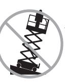
Do not raise the platform unless the machine is on a firm, level surface.
