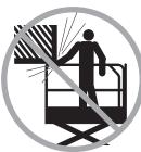
Be aware of crushing hazards when grasping the platform guard rail.
