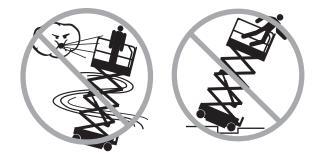
Do not drive the machine on or near uneven terrain, unstable surfaces or other hazardous conditions with the platform raised.
