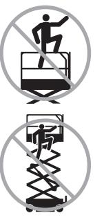
Do not sit, stand, or climb on the platform guard rails. Maintain a firm footing on the platform floor at all times.
