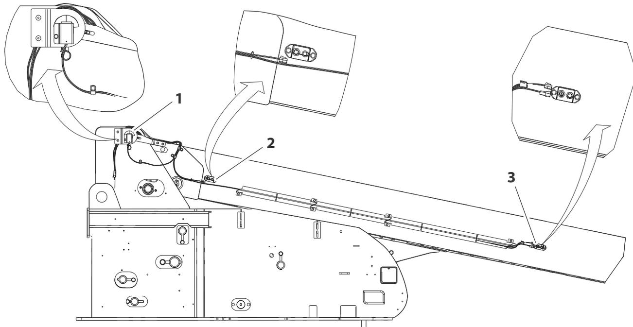
**Figure 2-2. Horizontal and Capacity Proximity Sensors- Sheet 1 of 2**
