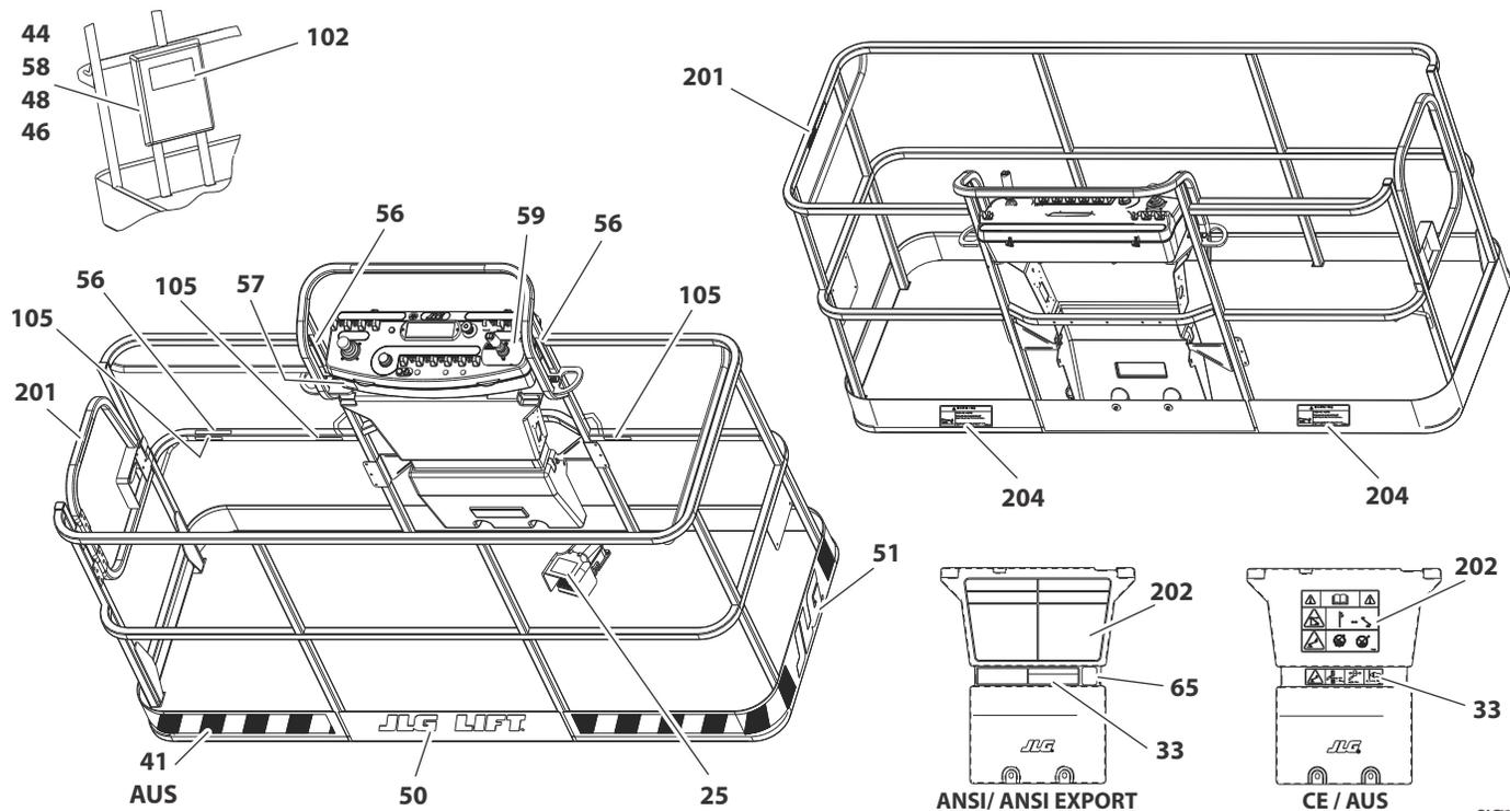
Figure 4-12. Decal Location - 800S Decal Location Sheet 5 of 5
