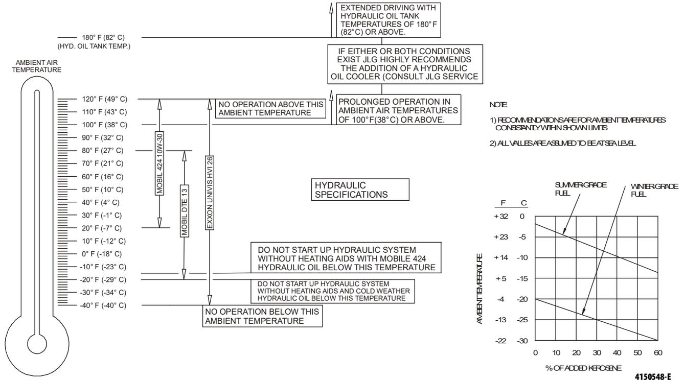
**Figure 7-3. Hydraulic Operating Temperature Specifications - Deutz - Sheet 2 of 2**
