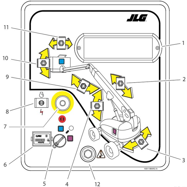
Figure 3-5. Ground Control Console - 860SJ with MSSO
