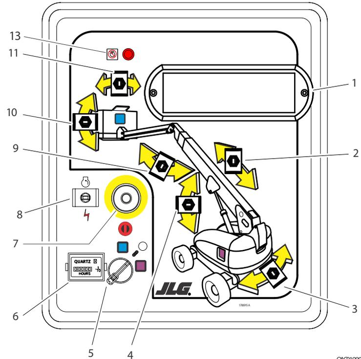
**Figure 3-4. Ground Control Console - 860SJ without MSSO**
