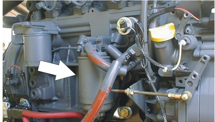
Lube Point(s) - Replaceable Element
