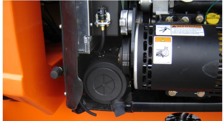
Lube Point(s) - Replaceable Element
