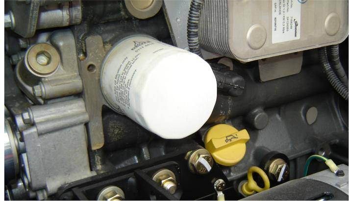
Lube Point(s) - Fill Cap/Spin-on Element
