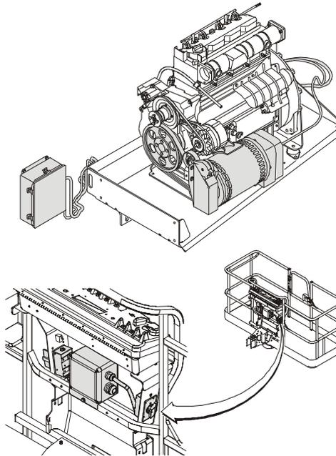
The SkyPower™ and generator systems supply AC power to the platform through an AC receptacle to run tools, lights, cutting, and welding equipment.
