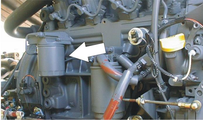
Lube Point(s) - Fill Cap/Spin-on Element
