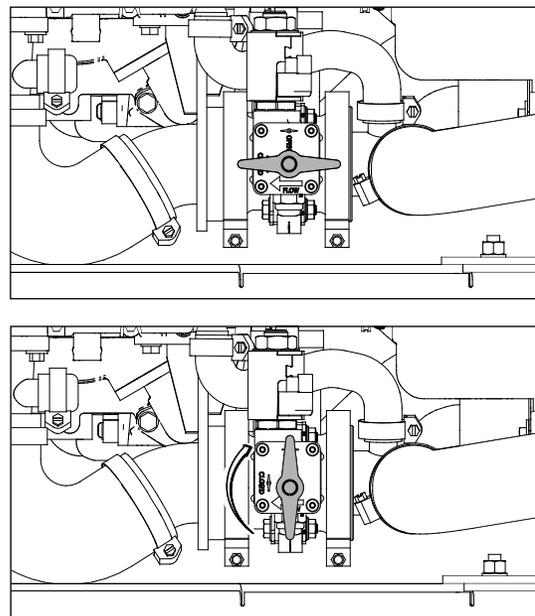
**Figure 4-3. ASOV Reset (Open to Closed Position)**
