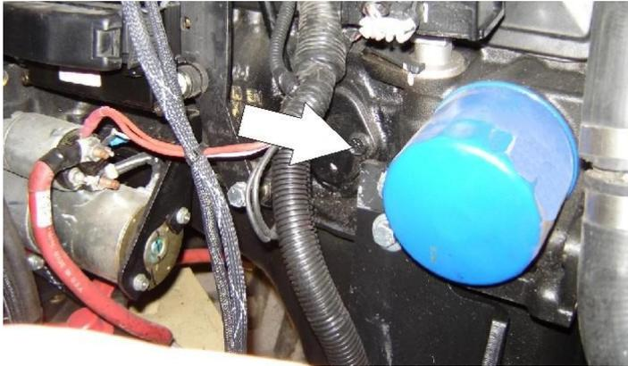
Lube Point(s) - Fill Cap/Spin-on Element
