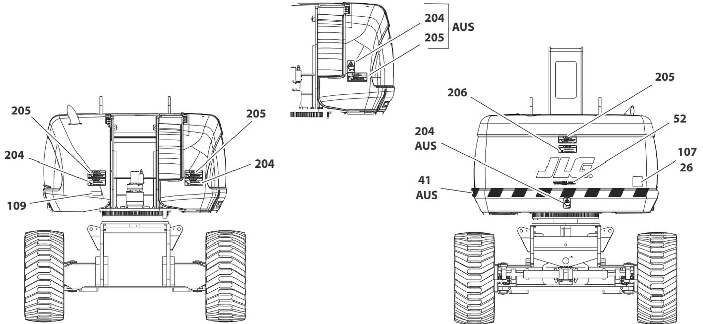
Figure 4-11. Decal Location - 800S Decal Location Sheet 4 of 5
