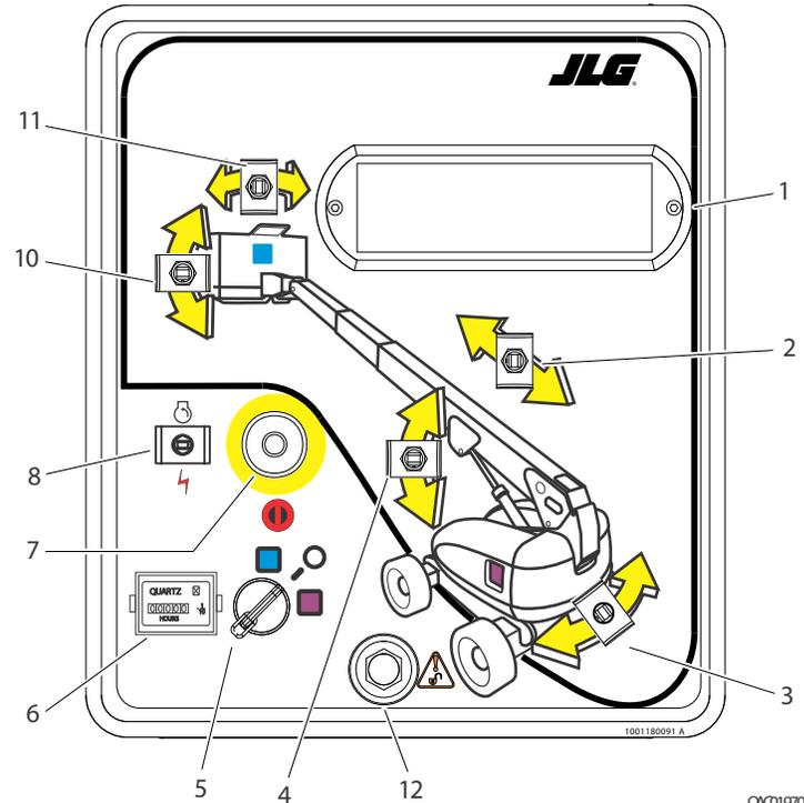
Figure 3-2. Ground Control Console - 800S with MSSO
