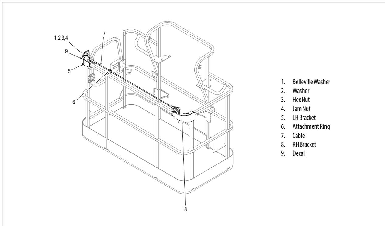
**Figure 6-2. Bolt-On External Fall Arrest System**
