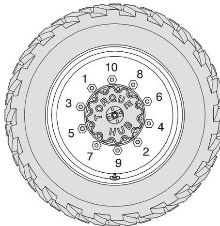
3. The tightening of the nuts should be done in stages. Following the recommended sequence, tighten nuts per wheel torque chart.
