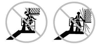
Be aware of crushing hazards when grasping the platform guard rail.
